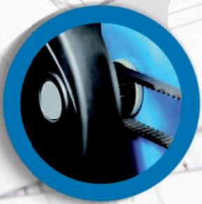
Cutting forward movement driven by a toothed belt transmission and wheel
