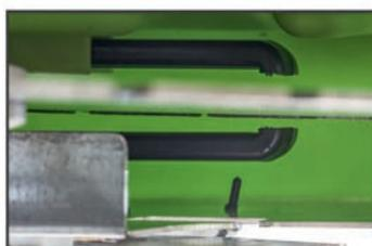
Cooling system for both blade sides.
