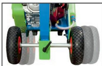
Rear tubeless puncture-proof wheels and adjustable axle.
