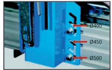
Height adjustable arm allows 3 blade sizes (**BALI 500 Mekano**).
